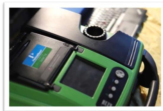
*Field portable Gas Chromatography-Mass Spectroscopy (GCMS) instrument used for pill testing at Groovin' the Moo.*
